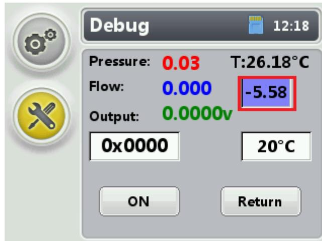
The **Pressure** value can be changed by changing the value in the red box, so as to complete the pressure sensor tuning. The setting range is -3.88 to -7.88. If the **Pressure** value cannot be adjusted to  $\pm 0.5$  within this range, this assembly may be installed improperly or damaged.
