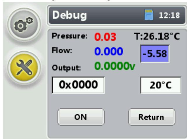
3. Rotate the control wheel to switch to the edit box (
