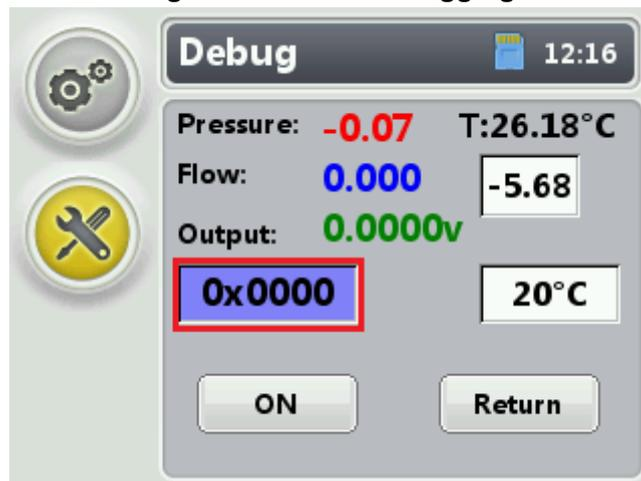
5. Connect the plug, click the ON button in the interface to turn it to OFF to start the motor. Any value of Pressure and Flow floating within normal range shows normal motor operation.
